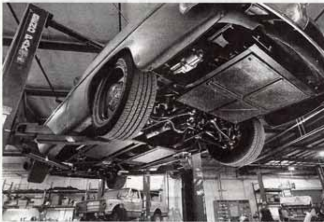
A 1949 Mercury Coupe EV is powered by Tesla batteries fitted throughout the car, including at the rear where the gas tank would normally be, for near-perfect balance.
