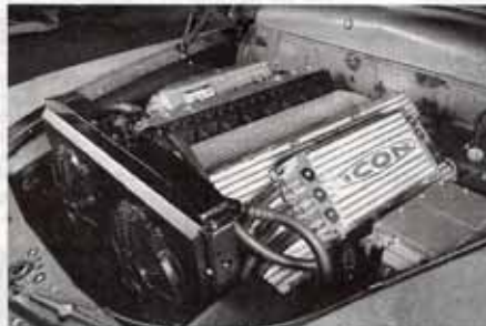
The engine bay is filled with electronics and batteries to give the 1949 Mercury Coupe the traditional V8 engine look.
